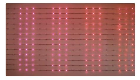
The CircuitPython LED Animation library includes pixel mapping helpers to make it super simple to treat a single LED strip as a grid. This is handy when you are using an LED matrix that is essentially one strip in series, or if you have a series of strips arranged in a grid. This section will go over the basics of the pixel mapping feature of the library and show you how to use it with animations.
