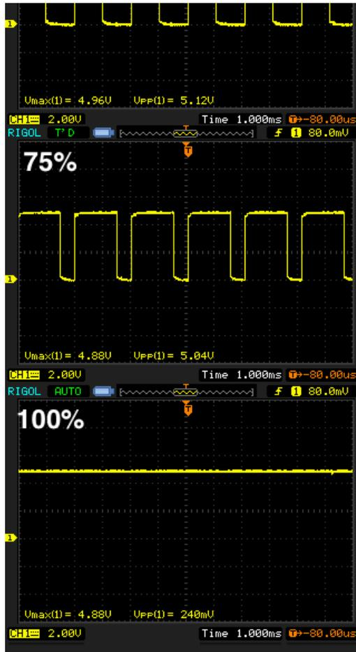
Back to controlling the LED, you can change the duty cycle by modifying the `pulseio.PWMOut.duty_cycle` (<https://adafruit.it/ySf>) attribute. Try setting the duty cycle to a 100% or fully on value with:
