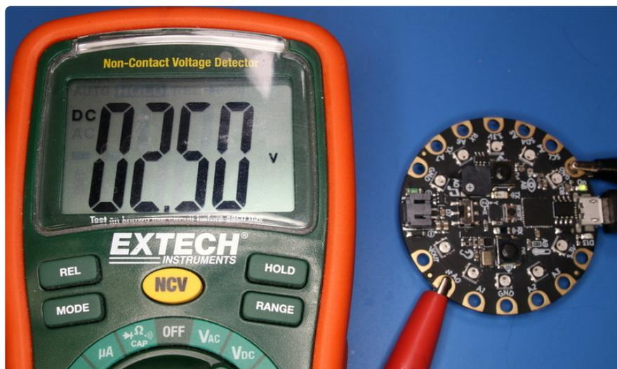
Just like with an analog input the digital to analog converter converts its digital value (the number like 10000) to a voltage based on an internal analog reference voltage. For the Metro M0 Express and Circuit Playground Express this reference voltage is 3.3 volts, so a value of 65535 means a full 3.3 volt output and a value of 0 means a 0 volt output. An in-between value will set a proportionally in-between voltage.
