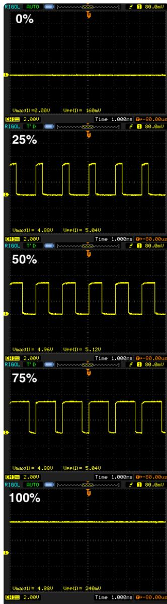
Back to controlling the LED, you can change the duty cycle by modifying the `pwmio.PWMOut.duty_cycle` (<https://adafru.it/ySf>) attribute. Try setting the duty cycle to a 100% or fully on value with:
