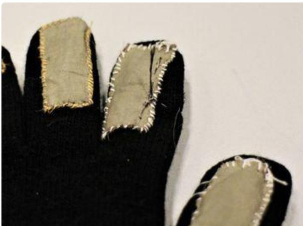
If you have a multimeter, check continuity between the CPX pins and the conductive thread pads.
