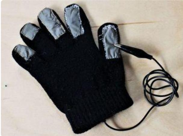
Use an alligator clip or insulated wire to connect the CPX ground ("GND") to the thumb pad.
