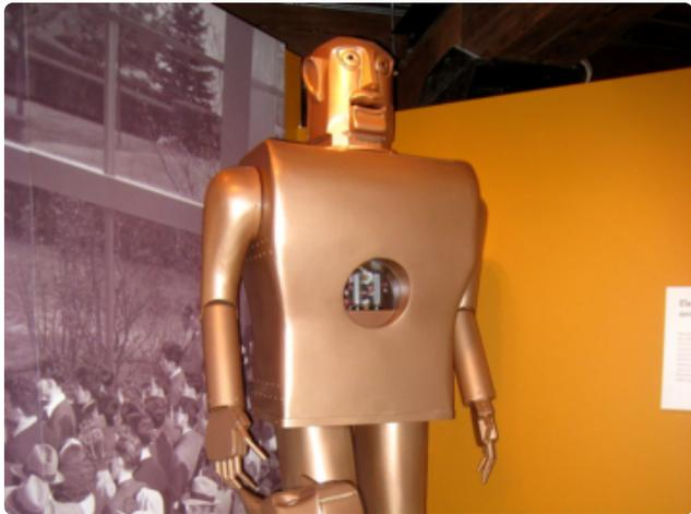
Elektro is the nickname of a robot built by the Westinghouse Electric Corporation in its Mansfield, Ohio facility between 1937 and 1938. Seven feet tall (2.1 m), weighing 265 pounds (120.2 kg), humanoid in appearance, he could walk by voice command, speak about 700 words (using a 78-rpm record player), smoke cigarettes, blow up balloons, and move his head and arms.
