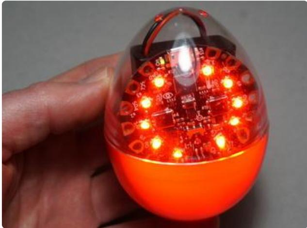
Here's the second egg with the Circuit Playground and the 3 x AAA battery pack installed. Good to go!
