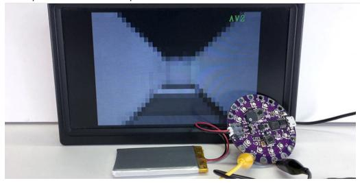
The DAC is *just* fast enough to generate low-resolution **composite video** that can be viewed on a television or monitor with composite video input (typically a yellow **RCA connector**).
