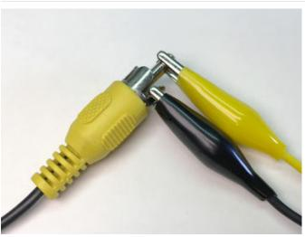
At the other end, connect AO to the "tip" (center) of the composite video connector, and ground to the "ring" (outside).
