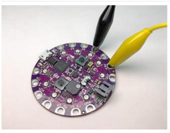
Connect a couple of test leads to **pin A0** and any **ground** pin.
