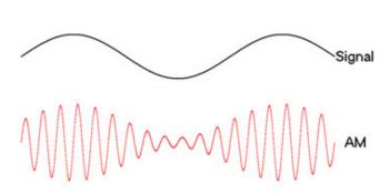
Amplitude modulation (AM) — the earliest method of sound transmission over radio — conveys a relatively low-frequency variable audio wave (such as voice or music, up to a few kilohertz) into a much higher fixed-frequency radio wave (500 KHz or more), called the carrier wave, by...you guessed it...modulating the amplitude of the carrier wave in direct proportion to the sound wave's shape.
