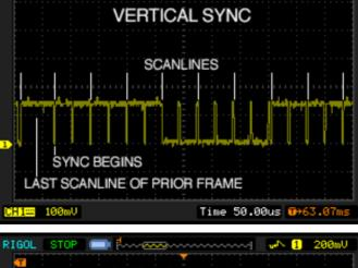
NTSC video runs at 29.97 frames per second. Each frame is comprised of 525 horizontal scanlines. Each scanline starts and ends with carefully-timed synchronization signals, with image data in-between: an analog voltage from about 0.3 to 1.0V determines the brightness at that point along the scanline.
