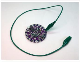
Clip a test lead or connect a length of wire to **pin A0** as a makeshift **antenna**. Just one end...the other is left unconnected. This is far from an optimal antenna, but we need *something* there.
