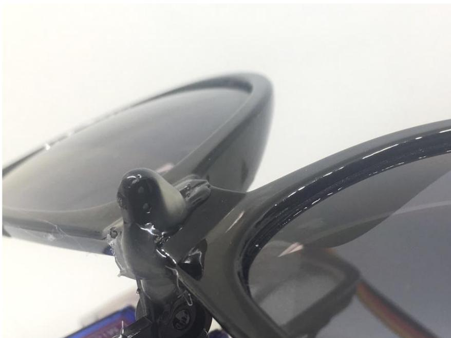
You need to mount the servo onto the top of the glasses frame. There are so many shapes and sizes that no universal instructions can apply. You will have to figure out how to attach the servo to the particular frames you have. In this case, the frames were metal and thin enough to slide into the slot in the servo's mounting bracket. Once more, hot glue does the job.
