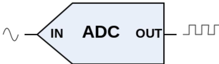
When you want to build a system that tracks an analog voltage, you need an Analog to Digital Converter (ADC) so your microcontroller or computer can read and record the results. If you want good measurements, you pick an ADC with the highest resolution you're willing to pay for, right?
