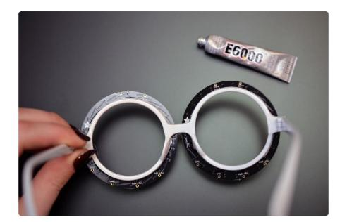
If you can glue the NeoPixel rings to the frames without covering the connections on the PCB, go for it. This will make it easier to make tidy wire connections. Hot glue is ok for now, but if you can permanantly affix them with E6000 or epoxy, go for it. Invest in a sturdy platform that won't fall apart during the subsequent steps.
