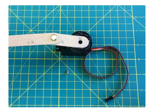
You can secure the servo horn to the servo shaft with the small screw and a screwdriver.
