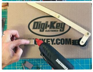
Place two more piece of cardboard like guide rails on the upper and lower "walls" of the stack. These should guide the slider, but not impede its motion.
