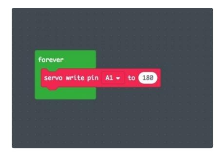
With the servo attached to power, ground, and pad **A1** on your Circuit Playground Express, download the program, connect the CPX to your computer over USB, press the reset button to enter bootloader mode. Then drag the downloaded .uf2 file to the CIRCUITPY drive.
