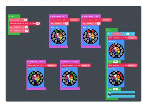
Using MakeCode, we'll create a program to control the slider crank. We'll give it two modes -- automatic and manual. In automatic mode, the servo will oscillate back and forth between extended and retracted positions on the slider
