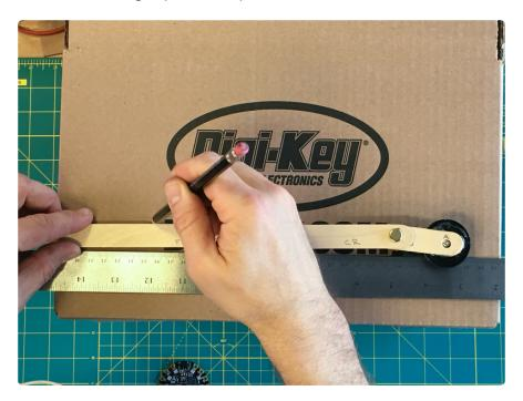
These two marks are where you will build up a small cardboard platform the rest the slider, and then two walls of cardboard for the upper and lower guides.
