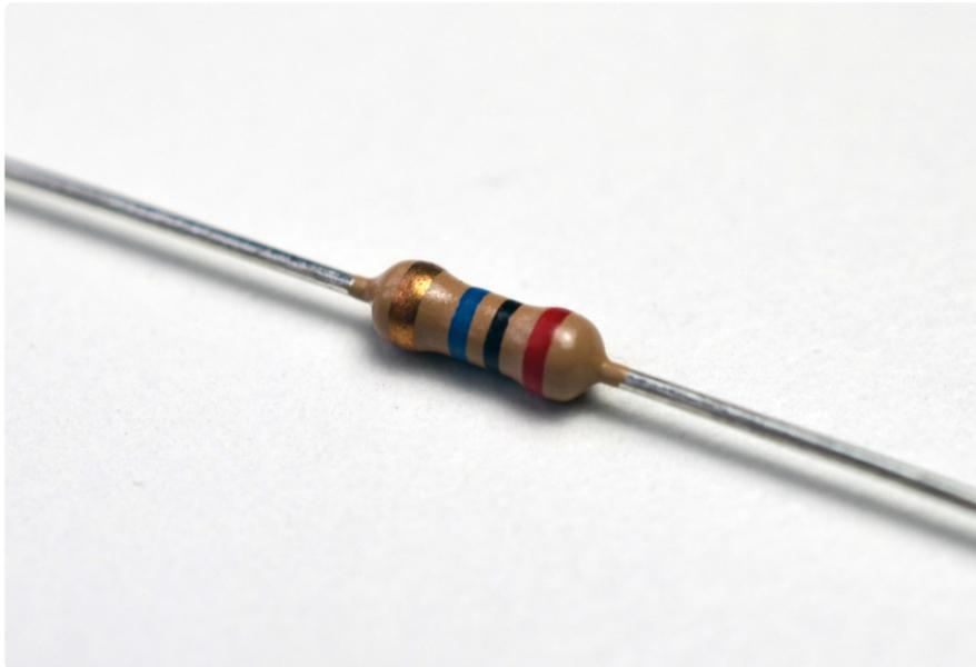
You'll also need a few very high resistors, 50K - 50M. The resistor value affects the sensitivity of the touch sensor-- at the low end the sensor will only be activated by absolute touch, and on the high end the sensor can be activated from a distance of 12 inches or more.
