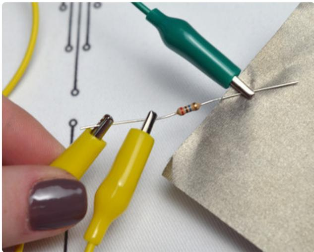
Clip yet another alligator to the non-fabric side of the first resistor. This extends the connection from D9 to the new conductive fabric pad.
