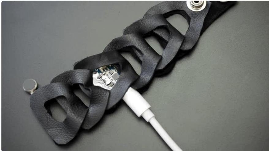
Load up the following code on Arduino GEMMA using the Arduino IDE. It should buzz the motor once per minute. If it's working, then adjust the interval variable to your desired number of seconds and reload the code.
