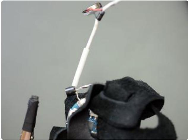
Solder the motor/diode assembly to the transistor's remaining pin (collector) and GEMMA Vin. The diode leads travel around the next link in the chain, concealing and protecting the circuit.
