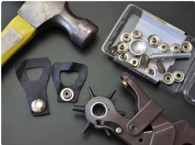
Use a snap setting tool to attach the snap parts, or use velcro tape instead.
