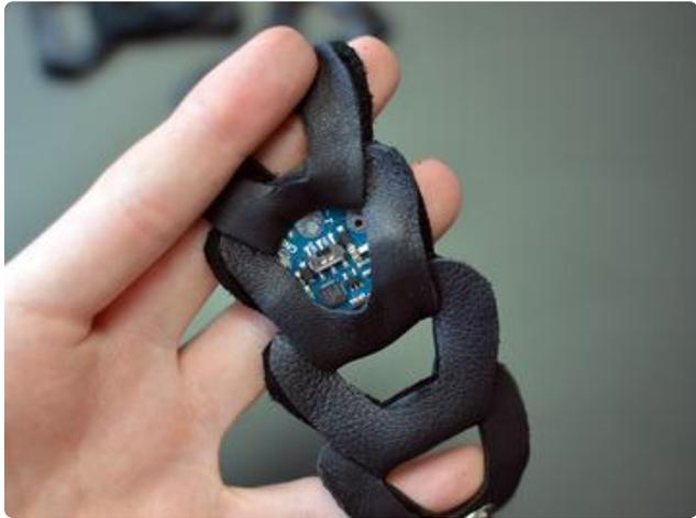
GEMMA fits snugly between the layers, which expose the power switch but hide the USB connector and JST battery connector. Slide GEMMA in from the side, with digital pin 1 facing towards the working end of the chain.
