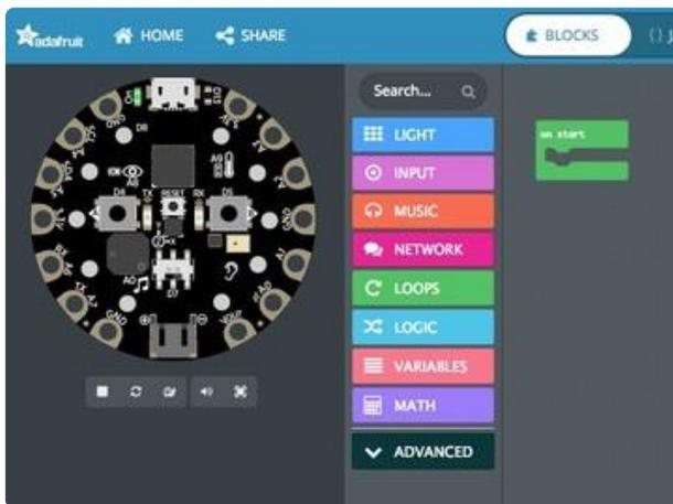
We soldered our light strand to pin A1. Tell the code by adding an `on start` loop (Loops > `on start`). This block will run ONCE when the board powers up, so it's the perfect place to define our setup.
