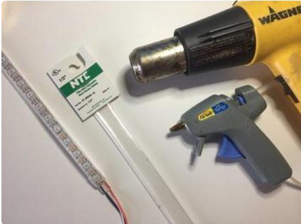
Cut four pieces of 1/4" clear heat shrink and place them over the end of each strip. Before you shrink them down, squirt some hot glue onto the strand to cover the solder connections. Then while the glue is still wet, use a heat gun to shrink the heat shrink down. This will create an indestructible and waterproof seal for your LED strips.
