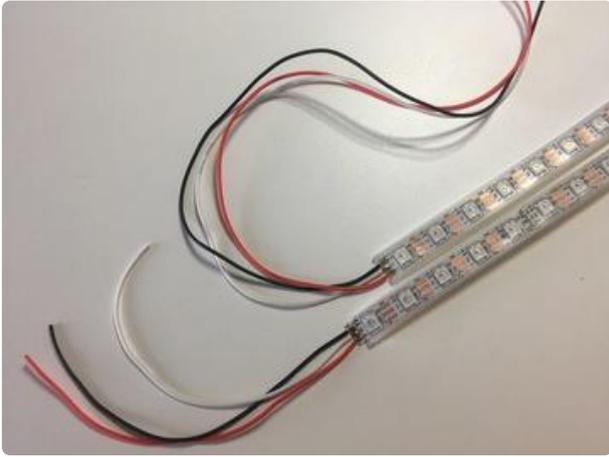
Find the "in" end of each cut strip (the arrows should be facing AWAY from that end). Solder 3 color coded wires to each strip: red to 5v, black to G, and white to IN.
