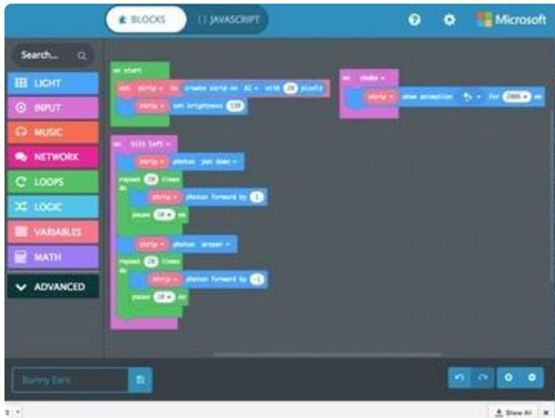
Get another instance of `(strip) photon (pen down)`. The quickest way to do this is to click on the block and copy it to your clipboard, and then paste it into your workspace (ctrl-c, ctrl-v). Change `(pen down)` to `(eraser)`. From here you can drag it below your loop function within the `on (tilt left)` block.
