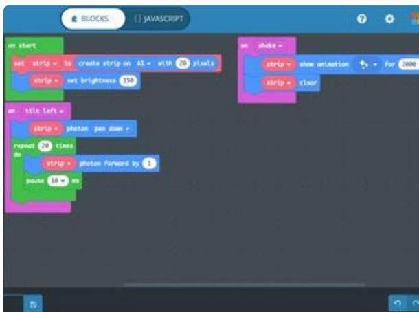
From the "Loops" bin, drag a **repeat (4) times** block inside the **on (tilt left)** block. Change the **(4)** to the number of neopixels in ONE strip (I have 20).
