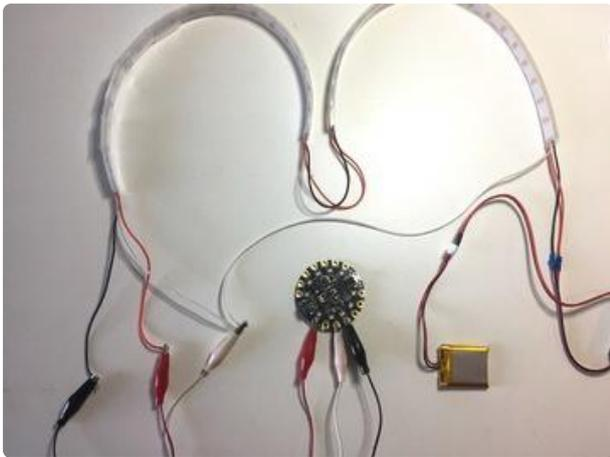
Solder a 4" red and black wire from the OUT end of strip #1 to the OUT end of strip #2.
