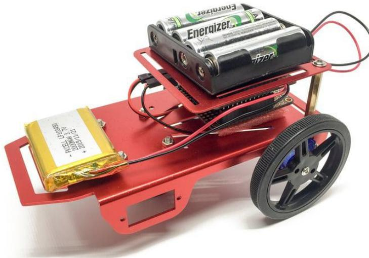
Note that on the last picture, I already connected the 3.7V LiPo battery to the ESP8266 feather board. However, you can wait until the robot is fully configured to connect the battery.
