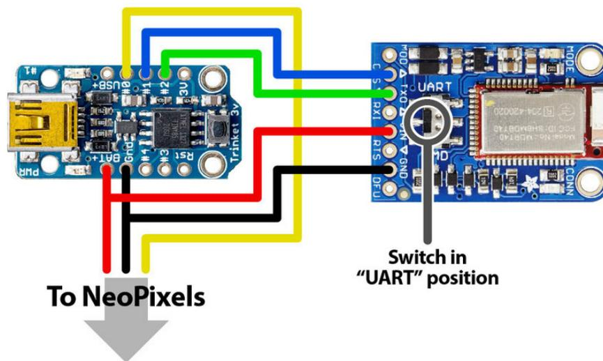
The switch on the Bluefruit LE UART Friend should be in the “UART” position.
