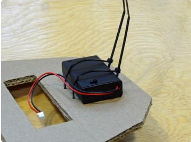
Put the batteries into the holder and slide the cover closed. Place the battery holder on the back side of the paddle as shown. Check to see that the on-off switch is easily accessible.
