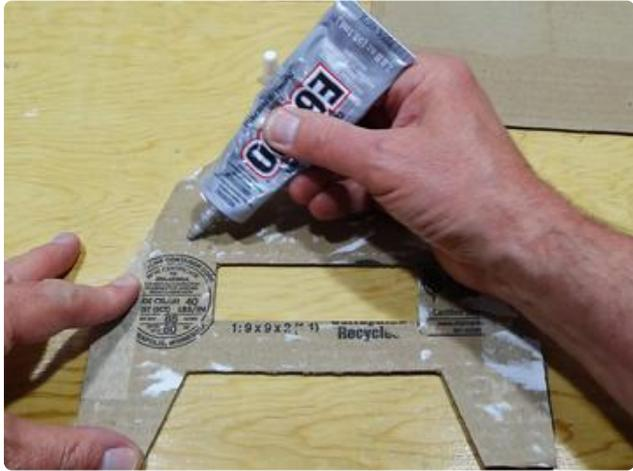
Peel the paper template off of the cut shape. We'll attach the cut cardboard to the remaining sheet using permanent adhesive.
