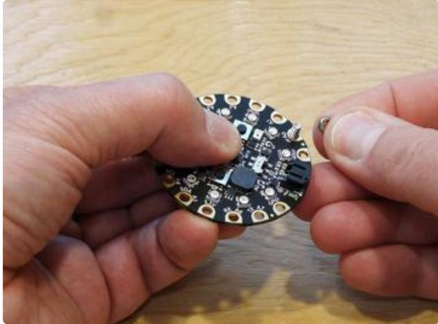
If you're planning on playing the Blues Playground through a guitar amplifier, now's a good time to add signal connectors to the CPX. We'll use alligator clips to connect to a guitar cable, so two screws will make that easier.
