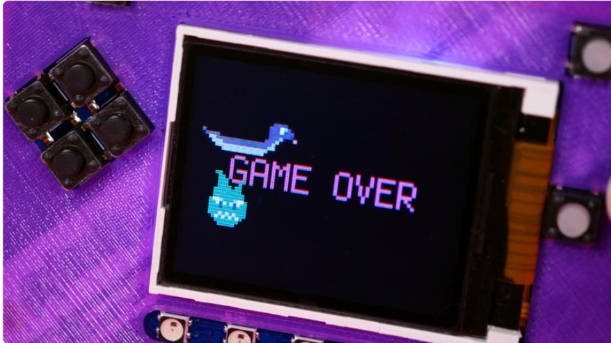
When you run out of game lives, the game goes into the `game_over` state. The Blinka and Sparky sprites freeze in their positions at the time of the final collision being detected, `"GAME OVER"` text is displayed in the center of the screen and three tones (a sad chromatic slide) play.
