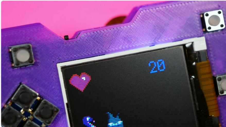
The `life_count` decreases by one every time that Blinka collides with a Sparky. This is detected when one of the Sparkys' `x` location is `8` and Blinka is slithering. When this occurs, the built-in speaker plays two tones (specifically a tritone, which sounds menacing) and `life_count` is updated to show the decrease.
