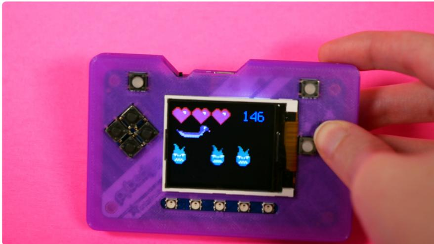
Blinka jumps every time the A button is pressed on the PyBadge board. To do this, when a button press is detected from the A button, the `snake` state is set to `False`. You'll remember that whenever the `snake` state is `True`, then the Blinka sprite is in the default slithering animation.
