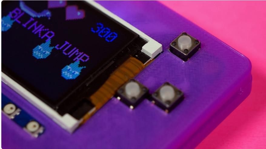
To start the game, you press the start button at the top of the PyBadge. When the game detects the start button is pressed, the game components are reset to their starting states. The three Sparky's are sent off screen, `life_count` is reset and the `new_game_text` is emptied.
