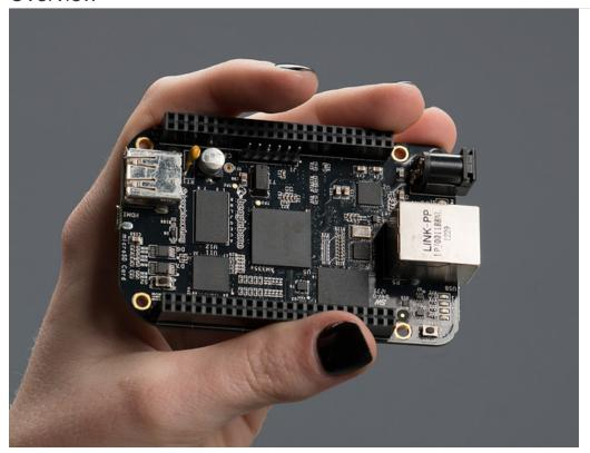
The BeagleBone Black includes a 2GB or 4GB on-board eMMC flash memory chip. It comes with the Debian distribution factory pre-installed. You can flash new operating systems including Angstrom, Ubuntu, Android, and others. The following pages will illustrate the steps to getting the latest of each type of supported distribution onto the on-board eMMC.
