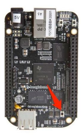
Hold the "User Boot" button down, and then plug in the power (USB or 5V adaptor). Keep holding down the button until you see the bank of 4 LED's light up for a few seconds. You can now release the button.
