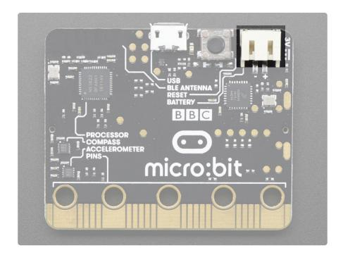
This little plastic connector is called a <u>JST PH connector</u> (https://adafru.it/yEQ). The battery pack that comes with the Go Bundle has the correct part to plug in there. The battery packs that Adafruit sell also come with the correct connector. Just plug and go.
