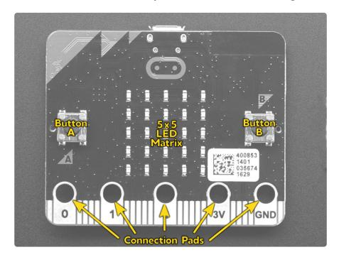
Along the bottom edge are a bunch of gold connection pads. The most important of these are the 5 bigs ones - the ones with the big holes. These will allow you to attach all kinds of additional items using alligator style clips. No soldering needed!
