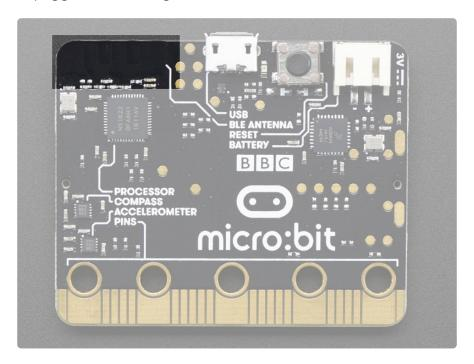
The actual hardware that does the Bluetooth communications is part of the main microcontroller (processor). This is just the antenna part, so maybe don't wrap that area in tinfoil or go drilling holes in it or something.
