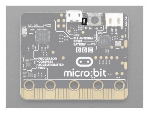
The status LED will NOT come on when powering via the battery jack. This is normal.
