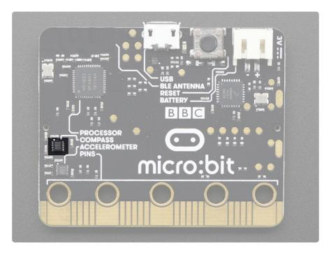
It's actually more like a magnet sensor. The Earth has a magnetic field that you can use to find North. However, anything else with a magnetic field will also be seen by the compass and can throw off the readings. Lot's of electrical devices generate magnetic fields, so you want to be sure and be away from them if you want to find out where North is.
