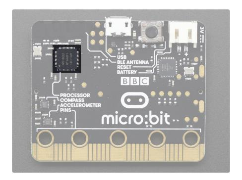
This particular microcontroller is made by a company called Nordic Semiconductor and has the cryptic name of nRF51822. Did some one say Nerf? Wah? Meh, it's just what they call it. It's probably 'n' for Nordic, and 'RF' for radio frequency or something. Don't worry about.
