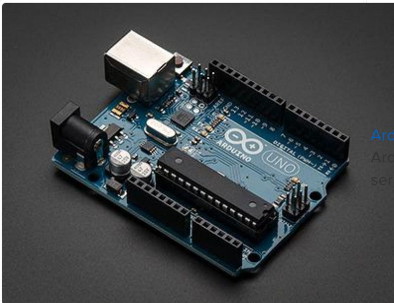
[Arduino Uno](#), [Micro](#), or other Arduino which supports USB serial and I2C communication.
