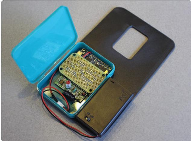
The circuit is mounted inside a plastic (not metal!) box (this one once held a bicycle tire patch kit). A piece of scrap plastic cut to size provides a base to which everything can be fastened with foam tape or hot glue...
