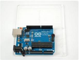
Remove the paper backing from the half size breadboard and stick it on next to the Arduino.
