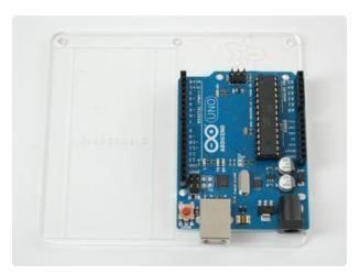
There are outlines showing how the Arduino and breadboard go on, make sure the print is right way up or it'll be confusing!
