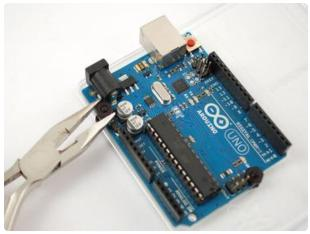
Attach the Arduino securely by screwing on the last two hex nuts
