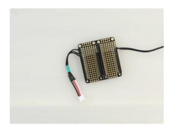
Soldered 3-pin JST cable
