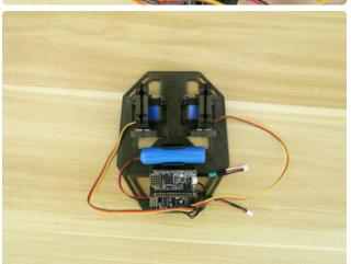
Install Battery to Back Plate Slide the 2200mAh battery into the battery holder through the side of the clip.
