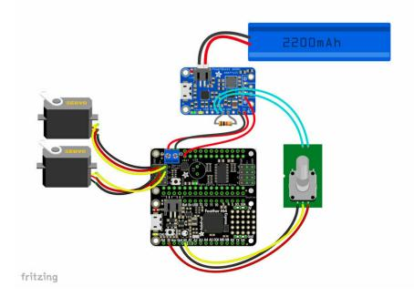
The diagram below provides a visual reference for wiring of the components. This diagram was created using the software package Fritzing (https://adafru.it/oEP).
