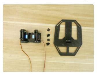
Hardware for Servo Mounts Use the following hardware to attach the servo mounts to the back plate.
