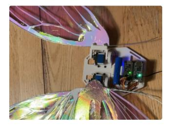
Insert your front-most wing into the wing mount and mark where the screw holes go. Poke through the holes with something sharp and insert two M3 15mm screws, and tighten down with their corresponding nuts.
