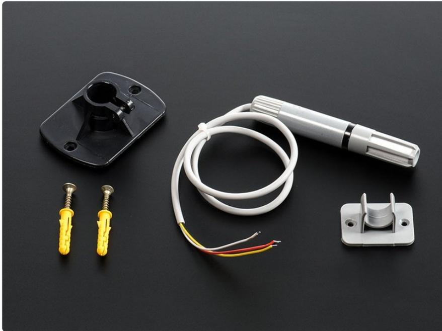
Finally we have an I2C-interface temperature & humidity sensor in a nice enclosed style. This sensor contains a thermistor temperature sensor and a capacitive humidity sensor. A small microcontroller inside does the readings and provides a simple I2C interface for reading the finished & calibrated output data. Especially nice is that this sensor is in a rugged case with mounting bracket, which makes it way superior to a normal PCB-mounted sensor.
