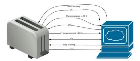
For example, you have an IoT AC unit that is monitored and controlled remotely. When you send a message for it to turn on you want to make sure it turns on! If you send a message and the transport fails, you can just keep sending messages over until you get a reply from the broker.
