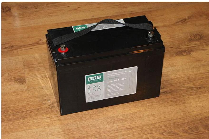
Lead Acid batteries ([image above](#) ()) are the workhorse batteries of industry. They are incredibly cheap, rechargeable, and easily available. Lead acid batteries are used in machinery, UPS's (uninterruptable power supply), robotics, and other systems where a lot of power is needed and weight is not as important. Lead acid batteries come in 2V cells, that means you can have a battery with an even number of volts. The most common voltages are 2V, 6V, 12V and 24V.
