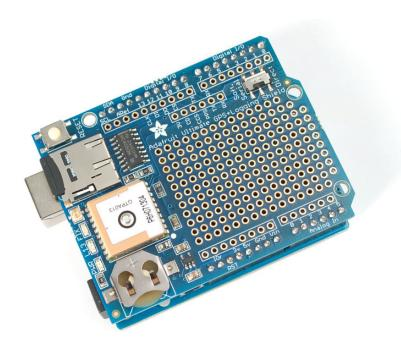
Each order comes with one assembled and tested shield, a stick of 0.1" male header and a 12mm coin cell. Some light soldering is required to attach the header to the shield in order to plug it into your Arduino. if you want to stack a shield on top, be sure to pick up a set of stacking headers to use instead.
