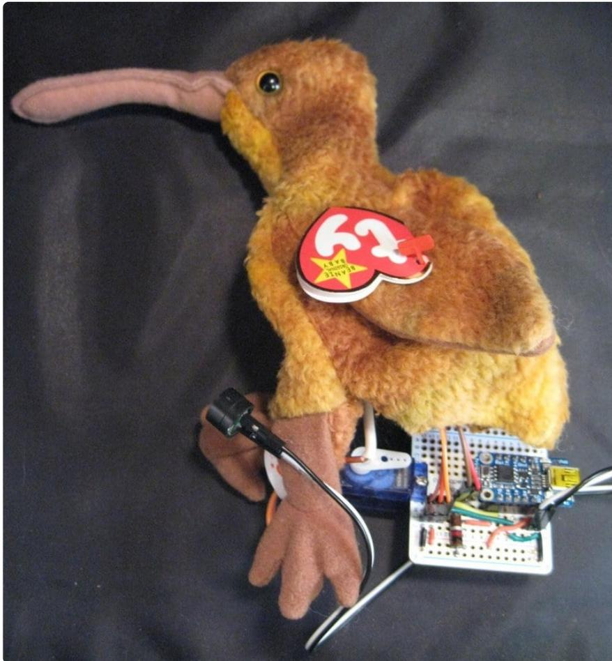
If you want to maximize the speaker sound, you can place it so the hole is exposed to the exterior of the animal. The fabric does not mute the chirp sound by much.
