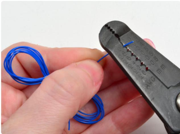
An antenna is required! We provide a 1meter long wire but you can also use a shorter or longer piece as desired. Strip a few mm from the end
