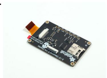
Carefully remove the display ribbon cable from the back of the display PCB.
