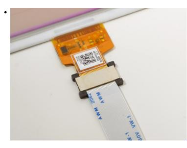
Plug in the 24-pin extension cable into the other end of the FFC/FPC extender.
