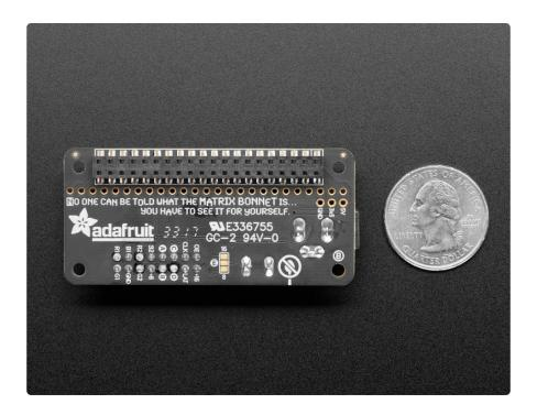
Works with any of our 16x32, 32x32 or 32x64 RGB LED Matrices with HUB75 connections (https://adafru.it/emd). You can also use 64x64 matrices by soldering a small jumper on the PCB (http://adafru.it/3649). Want more lights? No problem, chain multiple matrices together for a longer display - we've only tested up to 32x128 but it works just fine. The bigger the display the harder it is on the Pi, so keep that in mind if you're using a lower-powered Pi Zero.
