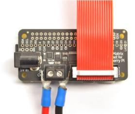
The RGB matrix also came with a 2x8 data cable. Connect one end to the matrix's INPUT side and the other end to the IDC socket on the HAT/bonnet.
