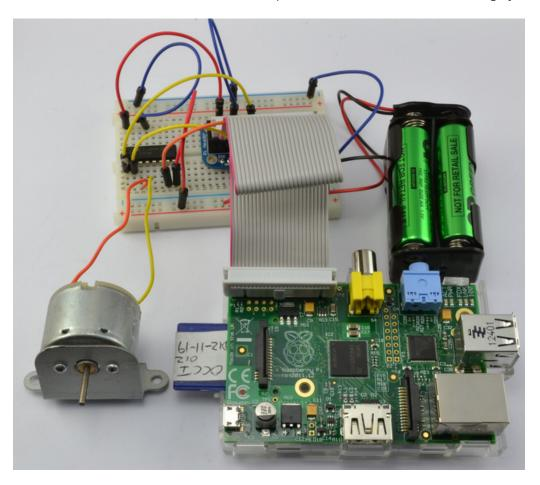
In Lesson 8, we used the Pi to generate pulses to control the position of a servo motor. In this lesson we use pulses to control the speed of a regular DC motor and the L293D motor control chip to reverse the direction of the current through the motor and hence the direction in which it turns.
