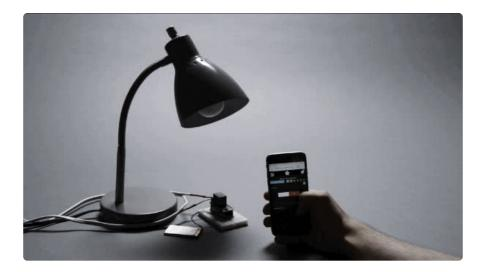
A Feather board without ambition is a Feather board without FeatherWings! This is the **Power Relay FeatherWing**. It gives you power to control, and control over power. Put simply, you can now turn on and off lamps, fans, solenoids, and other small appliances that run on up to 250VAC or DC power using any Feather board.
