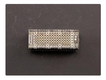
Solder the rest of the pins onto the PiCowbell.
