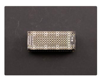
Solder the pins on each end of each socket header, so that the opposite four corners of the PiCowbell are soldered on.
