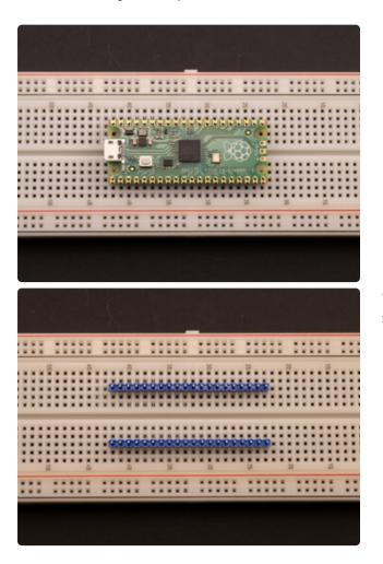
Use the Pico to line up the headers on a breadboard. This is the easiest way to ensure the headers are soldered on straight.
