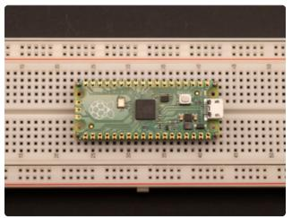
Solder the pins on each end of the two header strips, so the four corners of the Pico are soldered. This ensures the Pico and headers are attached properly while you continue to solder the rest of the pins.
