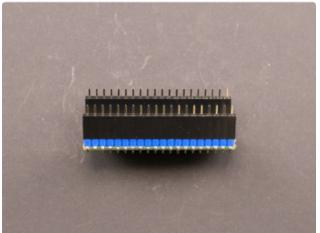
Place a standard-header-soldered Pico upside down on the table, so the long side of the header pins are facing up. Press the female sockets onto one of the rows of standard headers attached to the Pico, until both are fully attached.
