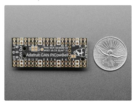
If you'd like to connect your Raspberry Pi Pico to a CAN Bus, the **Adafruit PiCowbell CAN Bus board** has a MCP2515 controller and TJA1051/3 transceiver! The controller used is the MCP2515, an extremely popular and well-supported chipset (https://adafru.it/18Be) that has drivers in Arduino and CircuitPython (https://adafru.it/18Bm)
