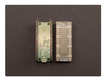
Ensure the PiCowbell is oriented correctly before beginning assembly. The PiCowbell should be top-down, so that you are looking at the bottom of the PiCowbell. The STEMMA QT connector should be on the same end as the Pico USB connector, and the reset button should be on the opposite end with the Pico debug pins.
