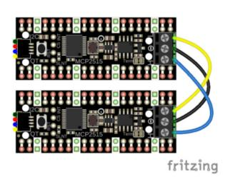
Once you have two Pico boards connected to CAN Bus PiCowbells, you can connect the CAN signals:
