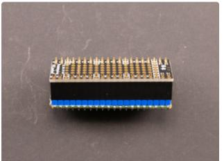
Press the PiCowbell onto the pins sticking up from the socket headers. You may need to push the stacking header pins in or out a bit to get the PiCowbell attached.
