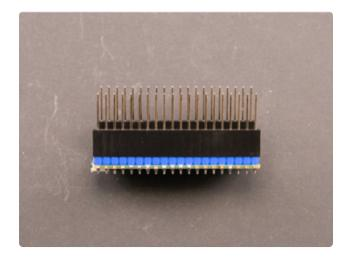
Place a standard-header-soldered Pico upside down on the table, so the long side of the header pins are facing up. Press the female sockets of each stacking header onto one of the rows of standard headers attached to the Pico, until they are fully attached.
