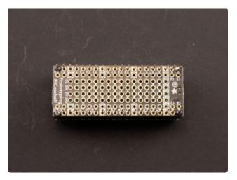
Solder the pins on each end of each stacking header, so that the opposite four corners of the PiCowbell are soldered on.
