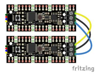
Once you have two Pico boards connected to CAN Bus PiCowbells, you can connect the CAN signals:
