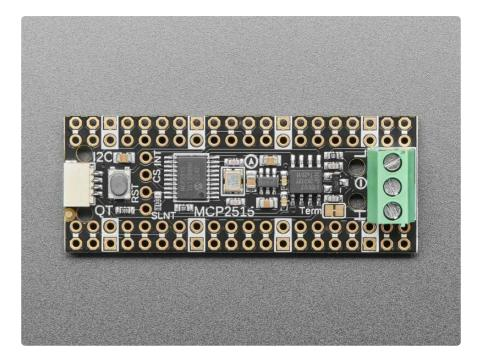
Ding dong! Hear that? It's the PiCowbell ringing, letting you know that the new Adafruit PiCowbell CAN Bus board is in stock and ready to assist your Raspberry Pi Pico (http://adafru.it/4864) and Pico W (http://adafru.it/5526) project in connecting to CAN bus networks for automotive or robotics projects.
