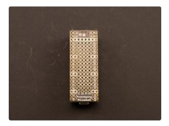
Press the PiCowbell onto the male pins sticking up from the stacking headers. You may need to push the stacking header pins in or out a bit to get the PiCowbell attached.
