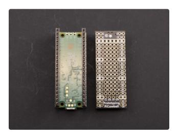
Ensure the PiCowbell is oriented correctly before beginning assembly. The PiCowbell should be top-down, so that you are looking at the bottom of the Cowbell. The STEMMA QT connector should be on the same end as the Pico USB connector, and the reset button should be on the opposite end with the Pico debug pins.
