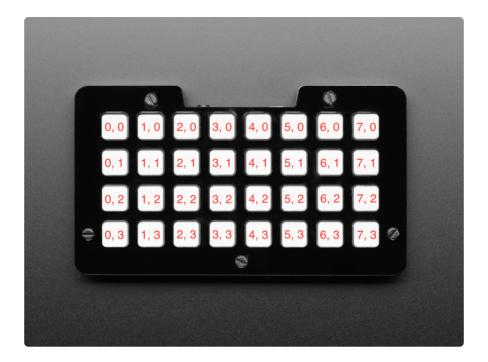
(0, 0) is always in the upper left corner and the rest of the grid follows standard positive (x, y) coordinates. So when the board is rotated 0 or 180 degrees, the board is oriented horizontally, and the lower right will be (7, 3).
