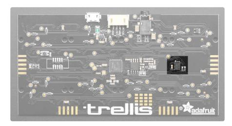
This sensor is on a separate I2C port, which is available in Arduino under **Wire1** or in CircuitPython under **board.ACCELEROMETER SCL** and **board.ACCELEROMETER SDA**
