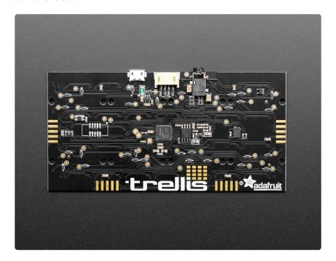
The native USB port can turn it into a MIDI USB device if you like - currently that's only supported in Arduino. Tether it to a computer or tablet, if you like. Or use it in standalone mode, as long as its powered from a USB power plug, it'll run whatever firmware is burned into it.
