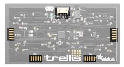
If you're using Arduino, the two GPIO are available on PIN\_WIRE\_SDA and PIN\_WIRE\_SCL for I2C usage, or A4 and A5 for analog reading.
