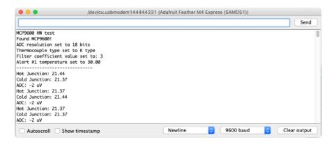
Note: The image above shows 9600 baud in the serial monitor. It should be 115200 to match the code!
