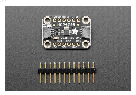
As of Aug 1, 2022 - we may make this board with the MCP4728 (default I2C address 0x60) or MCP4728A4 (default address 0x64). To check your board's I2C address, use either the <a href="Arduino"><u>Arduino</u></a> (https://adafru.it/10oD) or <a href="CircuitPython"><u>CircuitPython</u></a> (https://adafru.it/10oE) I2C scanner programs.
