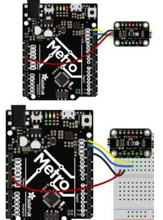
Arduino 5V to MCP4728 VCC (red wire) if you are running a 5V board Arduino (Uno, etc.). If your board is 3V, connect to that instead.
