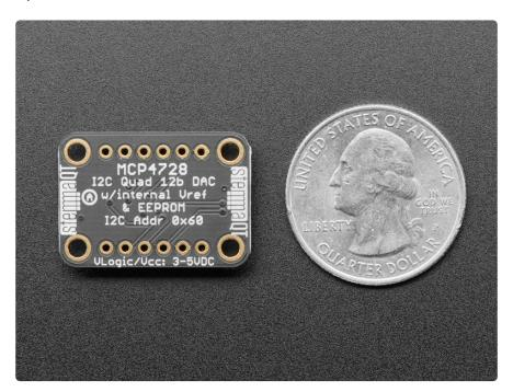
To take things even further, the MCP4728 lets you chose between two sources for your reference voltage: the input voltage that you use to power it on the VCC pin, or an internal 2.048V reference voltage. If you use the internal reference voltage (Vref in DAC speak) you can choose between 1X and 2X gain for the output, allowing your
