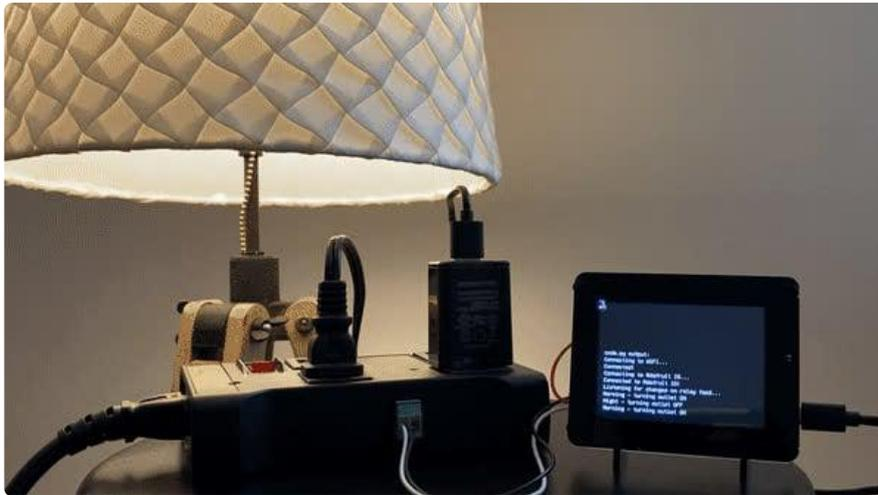
Every evening at 11PM, the scheduled trigger publishes the value "night" to your relay feed. The `on_battery_msg()` will read the new value, check if it matches the text "night", and turns off the outlet.
