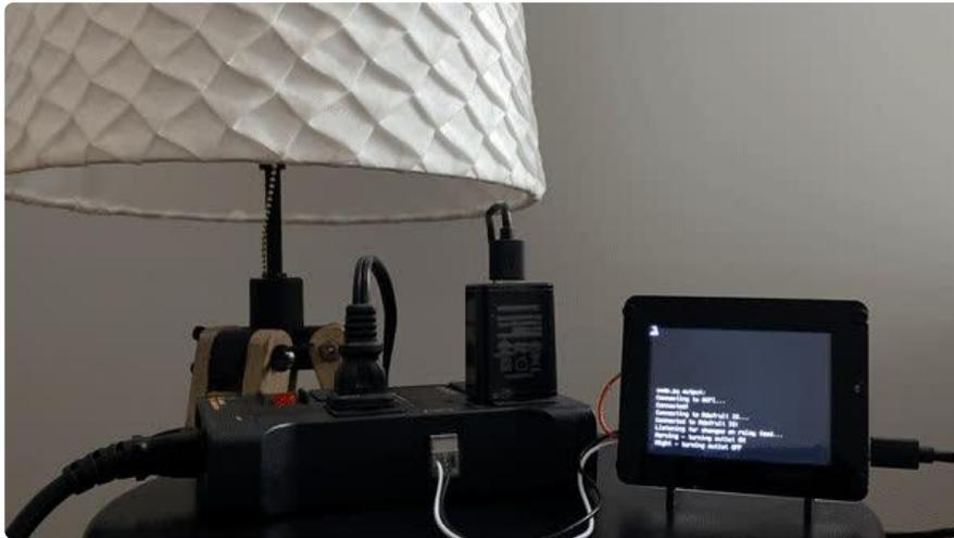
Add simple scheduling to your projects with an Adafruit IO schedule action. Turn on or off lamps, fans, solenoids, and other small appliances without the headache of reading and parsing output from real-time-clock (RTC) or obtaining the network time.
