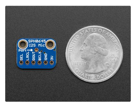
This I2S MEMS microphone is bottom ported, so make sure you have the hole in the bottom facing out towards the sounds you want to read. It's a 1.6-3.3V device only, so not for use with 5V logic (its really unlikely you'd have a 5V-logic device with I2S anyways). Many beginner microcontroller boards don't have I2S, so make sure its a supported interface before you try to wire it up!
