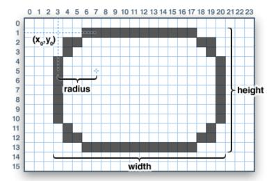
Here's an added bonus trick: because the circle functions are always drawn relative to a center pixel, the resulting circle diameter will always be an odd number of pixels. If an even-sized circle is required (which would place the center point between pixels), this can be achieved using one of the rounded rectangle functions: pass an identical width and height that are even values, and a corner radius that's exactly half this value.
