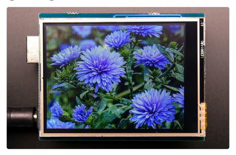
Loading .BMP images from an **SD card** (or the **flash memory chip** on Adafruit "Express" boards) is an option for most of our color displays...though it's not built into Adafruit\_GFX and must be **separately installed**.
