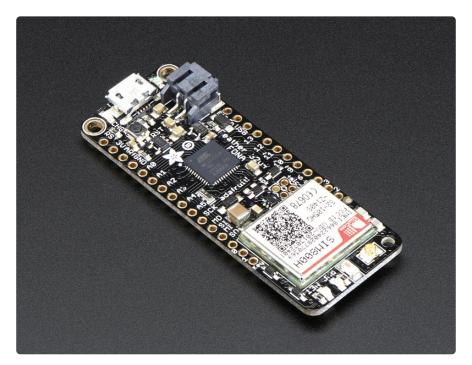
At the Feather 32u4's heart is at ATmega32u4 clocked at 8 MHz and at 3.3V logic, a chip setup we've had tons of experience with as it's the same as the Flora (http://adafru.it/659). This chip has 32K of flash and 2K of RAM, with built in USB so not only does it have a USB-to-Serial program & debug capability built in with no need for an FTDI-like chip, it can also act like a mouse, keyboard, USB MIDI device, etc.
