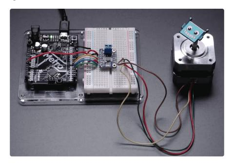
There's two digital inputs per H-bridge (one for each half of the bridge), you can PWM one of the inputs to control motor speed. Runs at 2.7V-10.8V logic/motor power. The motor voltage is the same as the logic voltage, but logic voltage from 2.7V or greater will work so no need to worry if you are powering the motors from 9V and using 3.3V logic. For higher voltages, check out the TB6612. (http://adafru.it/2448) For much higher voltages and currents check out the DRV8871! (http://adafru.it/3190)
