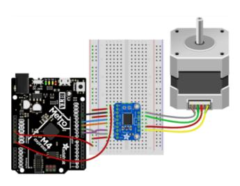
Board VCC to breadboard power rail
