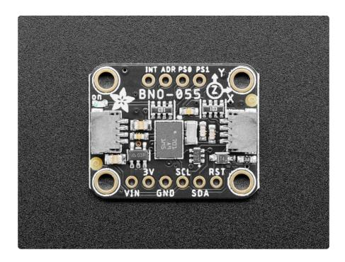
The new version of the board includes <u>SparkFun qwiic</u> (https://adafru.it/ Fpw) compatible <u>STEMMA QT</u> (https://adafru.it/Ft4) connectors for the I2C bus so you don't even need to solder! Use a a plug-and-play STEMMA QT cable to get 9 DoF data ASAP.
