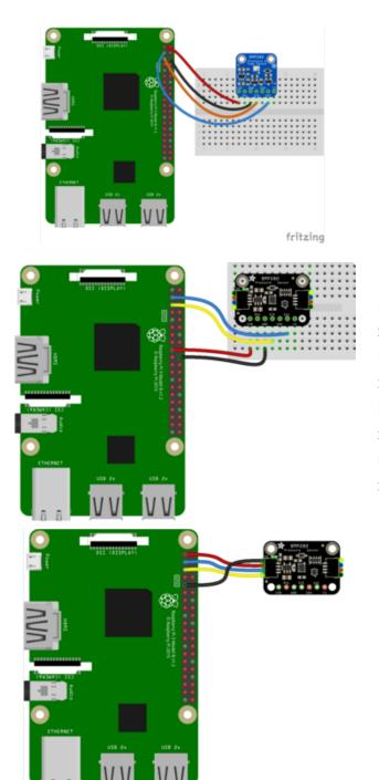
Pi 3V3 to sensor VIN (red wire on STEMMA version) Pi GND to sensor GND (black wire on STEMMA version) Pi SCL to sensor SCK (yellow wire on STEMMA version) Pi SDA to sensor SDI (blue wire on STEMMA version)
