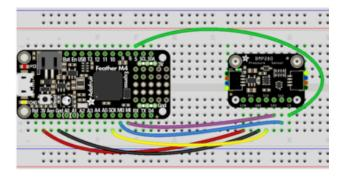
Board 3V to sensor VIN Board GND to sensor GND Board SCK to sensor SCK Board MOSI to sensor SDI Board MISO to sensor SDO Board D5 to sensor CS (or use any other free digital I/O pin)
