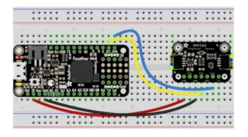
Board 3V to sensor VIN (red wire on STEMMA version) Board GND to sensor GND (black wire on STEMMA version) Board SCL to sensor SCK (yellow wire on STEMMA version) Board SDA to sensor SDI (blue wire on STEMMA version)
