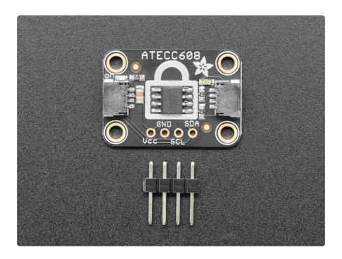
To make working with the ATECC608 as easy as possible, we've put it on a breakout PCB with the required support circuitry and <a href="SparkFun qwiic">SparkFun qwiic</a> (https://adafru.it/Fpw) compatible <a href="STEMMA QT">STEMMA QT</a> (https://adafru.it/Ft4) connectors. This allows you to use it with other similarly equipped boards without needing to solder. This chip will work with 3.3V or 5V power/logic micros, so it's ready to get to work with a range of development boards.
