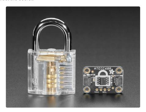
The ATECC608 is the latest crypto-auth chip from Microchip, and it uses I2C to send/receive commands. Once you 'lock' the chip with your details, you can use it for
