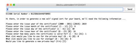
The ATECC608A will quickly generate a self signed certificate and display it on the serial monitor. It'll also include a SHA1 hash for verifying the certificate.
