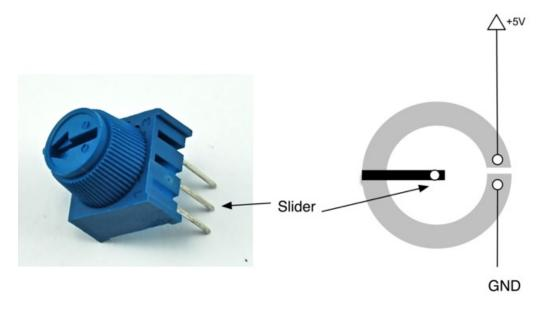
Your pot has a circular 'track' that acts as a resistor, in our case it's a 10 k $\Omega$  resistor. However, the difference with a pot, is that there is also a middle connection called the 'slider'. This connection is rotated when you turn the pot. So if you connect one end of the pot to 5V and the other to GND, then the voltage at the slider will vary between 0 and 5V as you turn it.
