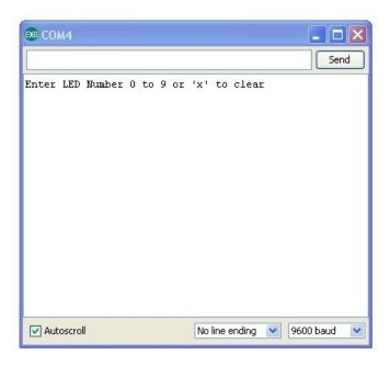
This window is called the Serial Monitor and it is part of the Arduino IDE software. Its job is to allow you to both send messages from your computer to an Arduino board (over USB) and also to receive messages from the Arduino.
