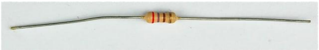
270 \Omega Resistors (red, purple, brown stripes) - you can use up to 1K ohm although it will be a little dimmer
