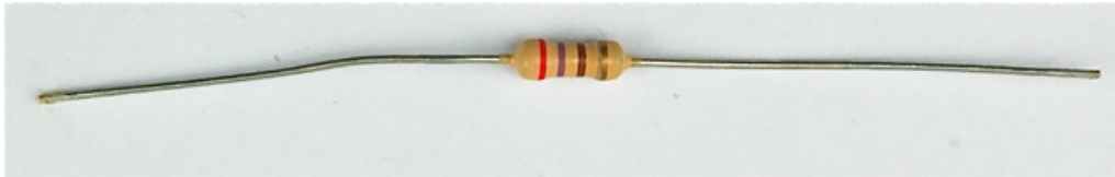
270 \Omega Resistors (red, purple, brown stripes) - you can use up to 1K ohm although it will be a little dimmer 3
