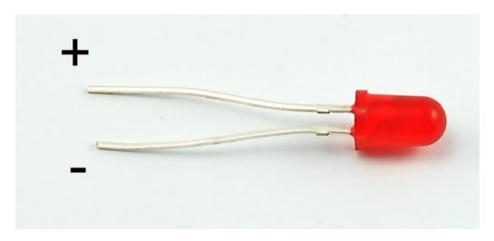
If you do not use a resistor with an LED, then it may well be destroyed almost immediately, as too much current will flow through the LED, heating it and destroying the 'junction' where the light is produced.
