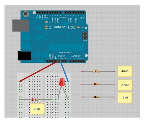
The Arduino is a convenient source of 5 Volts, that we will use to provide power to the LED and resistor. You do not need to do anything with your Arduino, except plug it into a USB cable.
